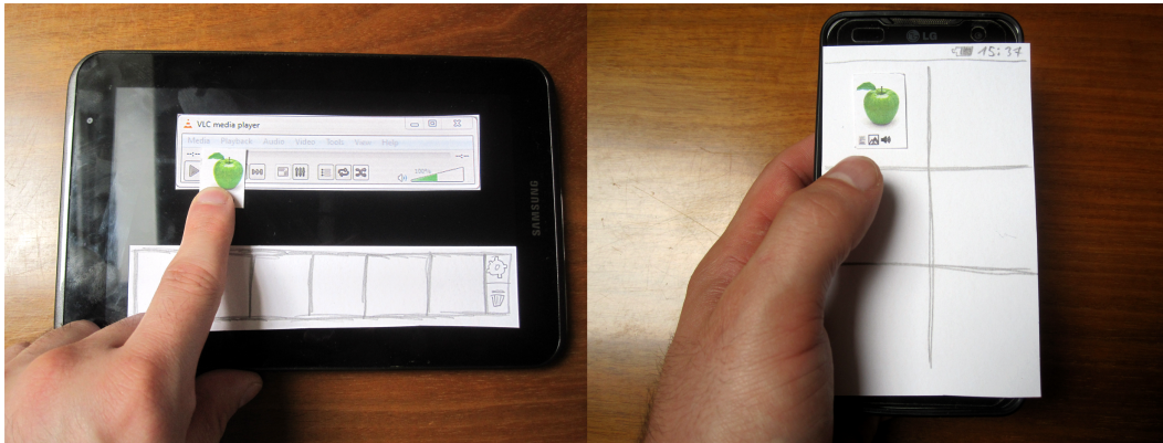
Figure 3.11: Photos of the paper prototype for mobile devices. On the left, a tablet is shown, experimentally using the Metamorph dock instead of the app. On the right, a smartphone featuring the Metamorph app is shown.
